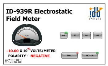
The ID-939R can be used in a stand-alone configuration or connected via a CAT5 Ethernet cable to a desktop or laptop computer for remote controlling. It is then possible to locate the equipment in a suitable environmental test chamber to control environmental parameters. A simple GUI (Graphical User Interface) is provided for controlling the instruments and storing test results.
