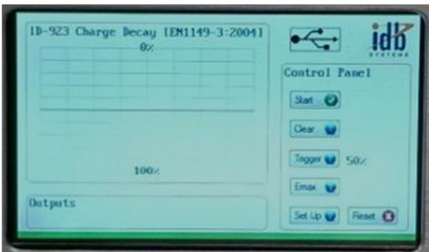
Charging of the test specimen is carried out by an induction effect and immediately under the test specimen, which is horizontally arranged, a field-electrode is positioned, without contacting the specimen, and a high-voltage is rapidly applied to the field-electrode.
