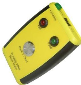
The unit is housed in a durable lightweight plastic moulded case with rubber hand grips on the side, making it ideal to use as a portable tester.
